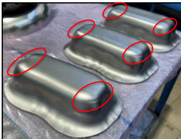
Residual issues with pole-forming, discarded ~15% of parts.
