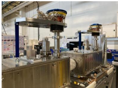
Assembly of RFD crab cavity module
