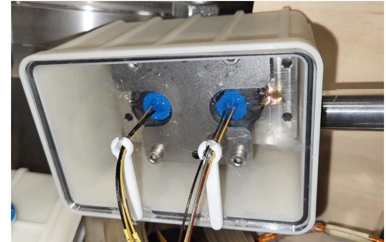
Cabling, jointing and potting on F1 bench
