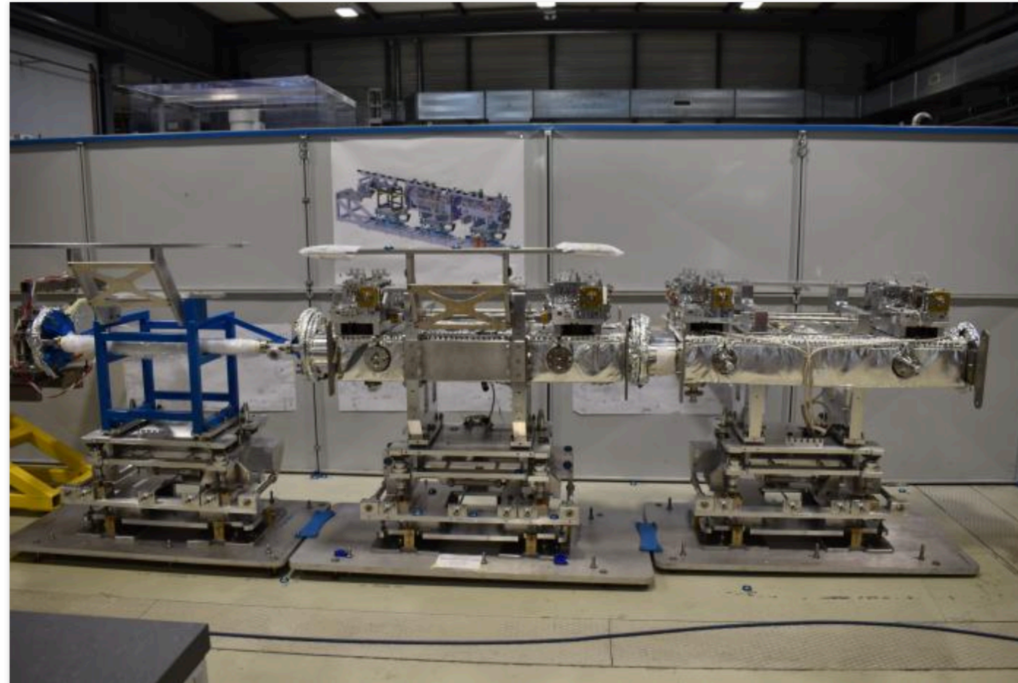
Collimator's prototypes together on the mock-up stand mock-up stand in building 927 (Image: Regis Seidenbinder)
