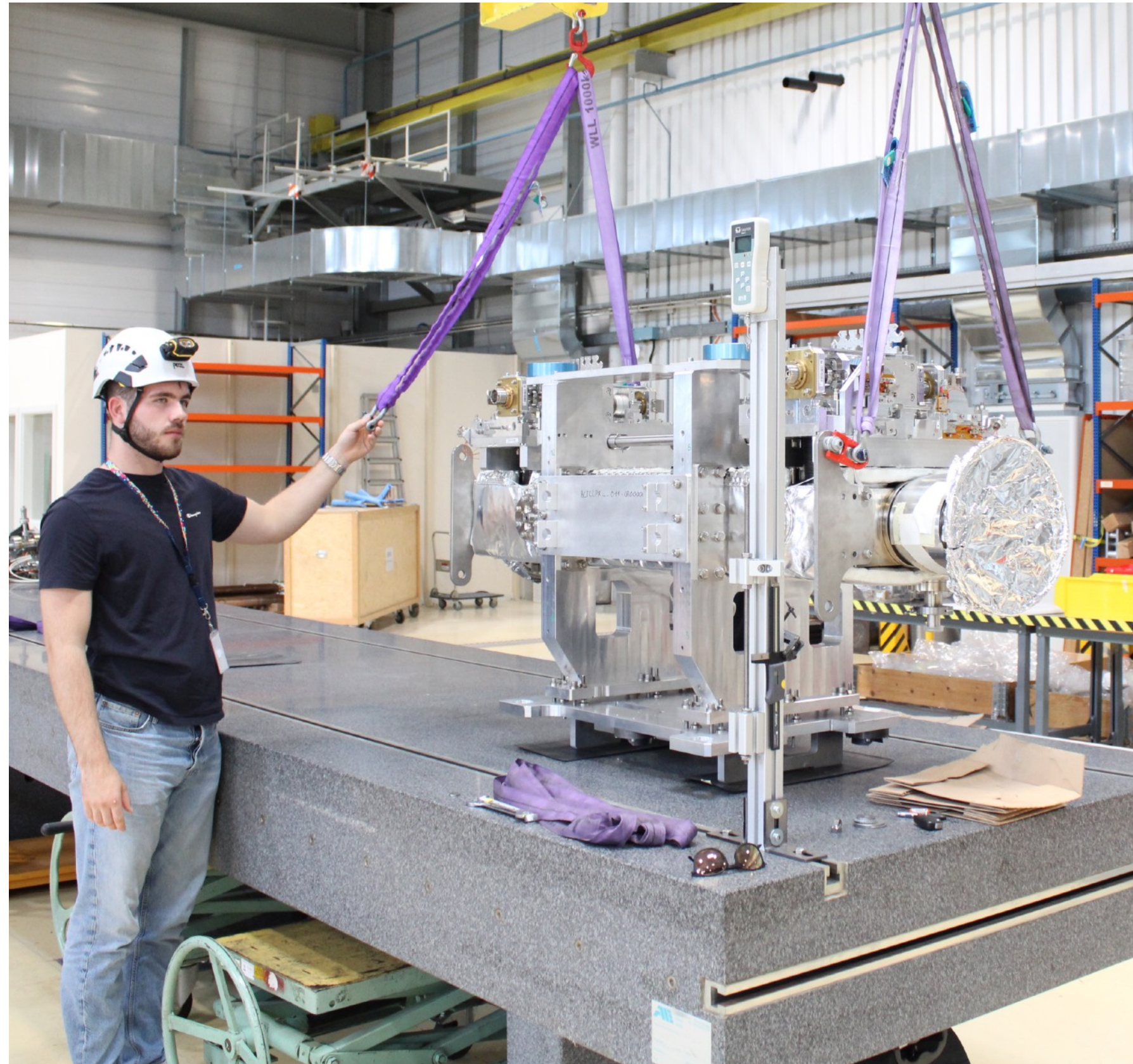
Installation of collimator on marble for flange flatness measurements.
