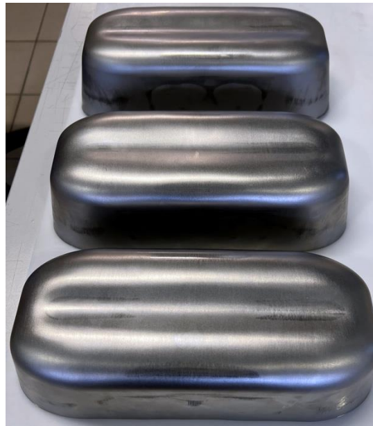
Unacceptable Poles (left) and Acceptable Poles (middle) from the same Niobium sheet. Difficult stamping of Waveguides (right)
