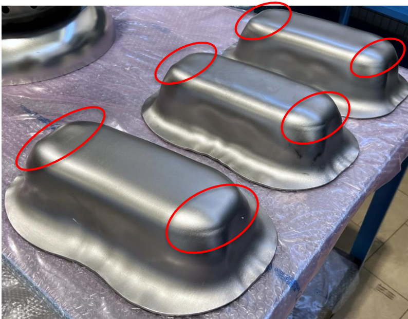
Unacceptable Poles (left) and Acceptable Poles (middle) from the same Niobium sheet. Difficult stamping of Waveguides (right)
