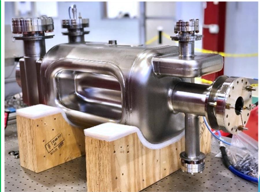
RF check of NRFDP002 without ancillaries (FNAL)
