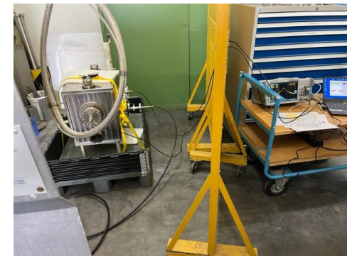
Pressure test with RF follow up
