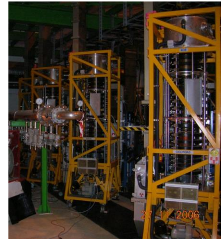
CERN LHC, 16 x TH 2167 klystrons in LHC UX45 cavern delivering 330 kW @ 400 MHz, into operation since 2008
