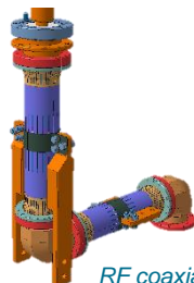
RF coaxial lines
