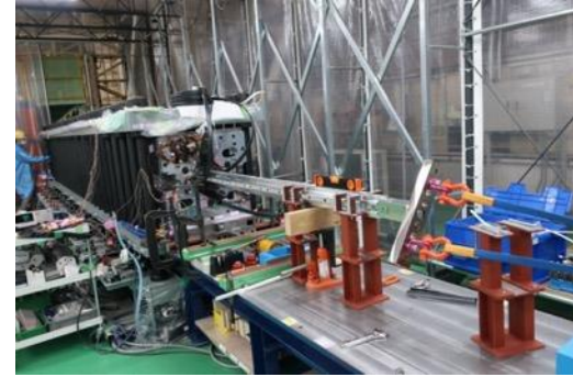
Removal of collaring mandrel
