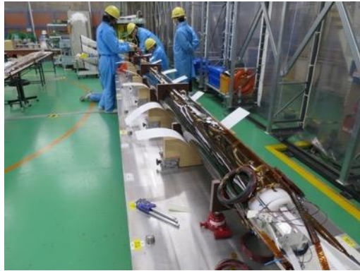
Top/bottom coil assembly
