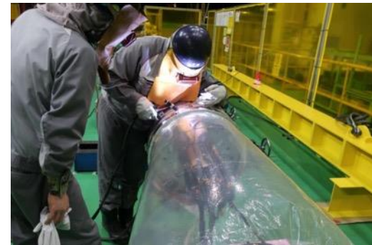
End ring welding
