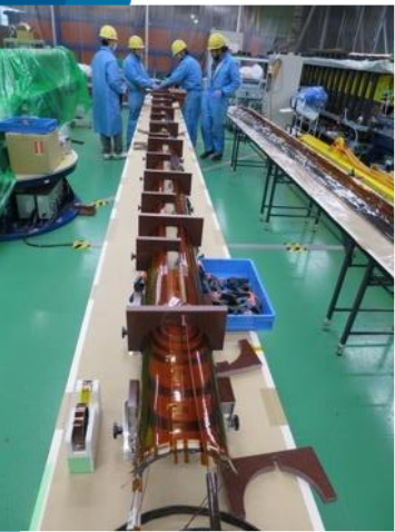
QPH, ground insulation wrapping
