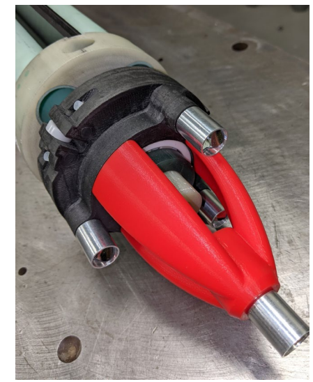
Laser tracker targets visible from non-drive end
