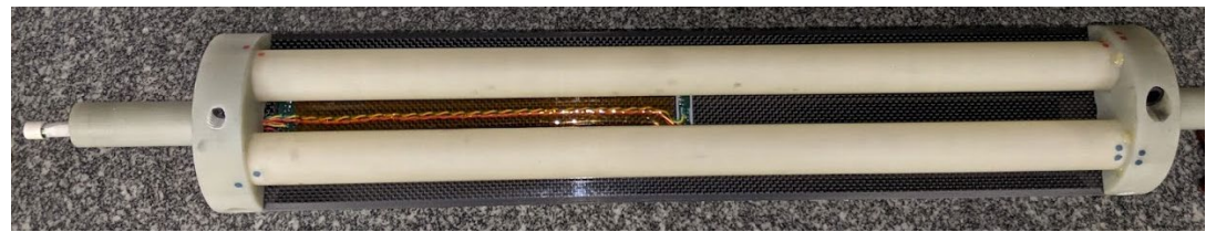
PCB probes stiffened with carbon fiber or G10
