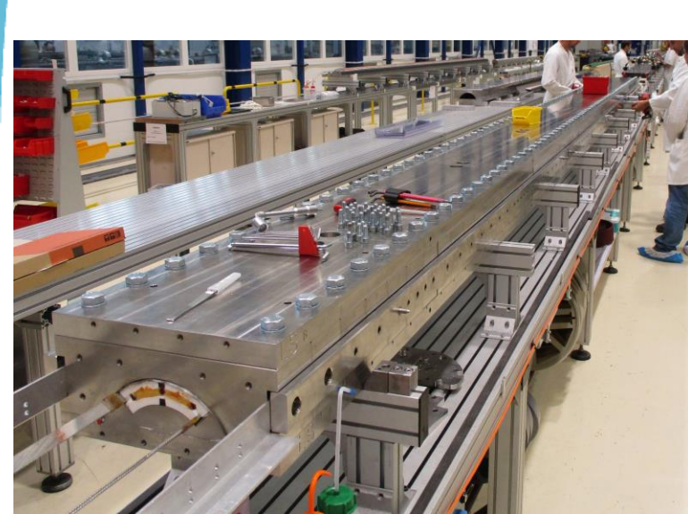
Coil closed in the impregnation fixture
