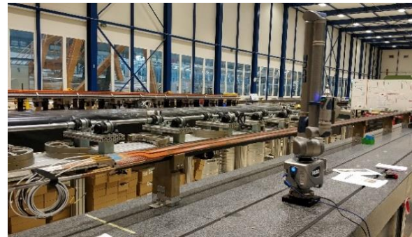
Metrology measurements of the impregnated coil
