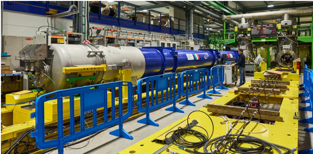
D2 prototype tested on bench C2 in direct connection. On the photo: Lucio performing magnetic measurements
