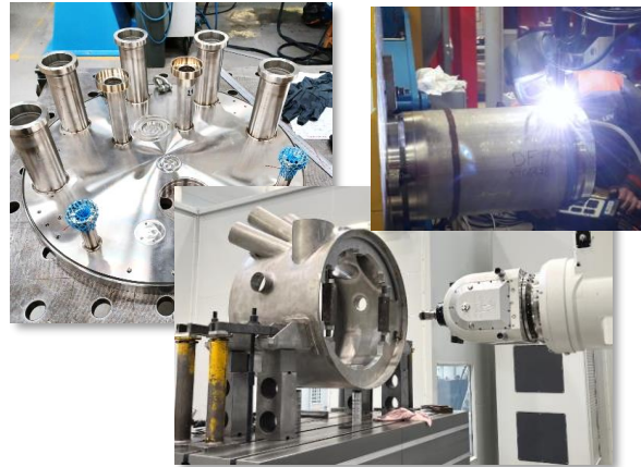
Manufacturing of DFHX prototype unit at CERN & RFR solutions
