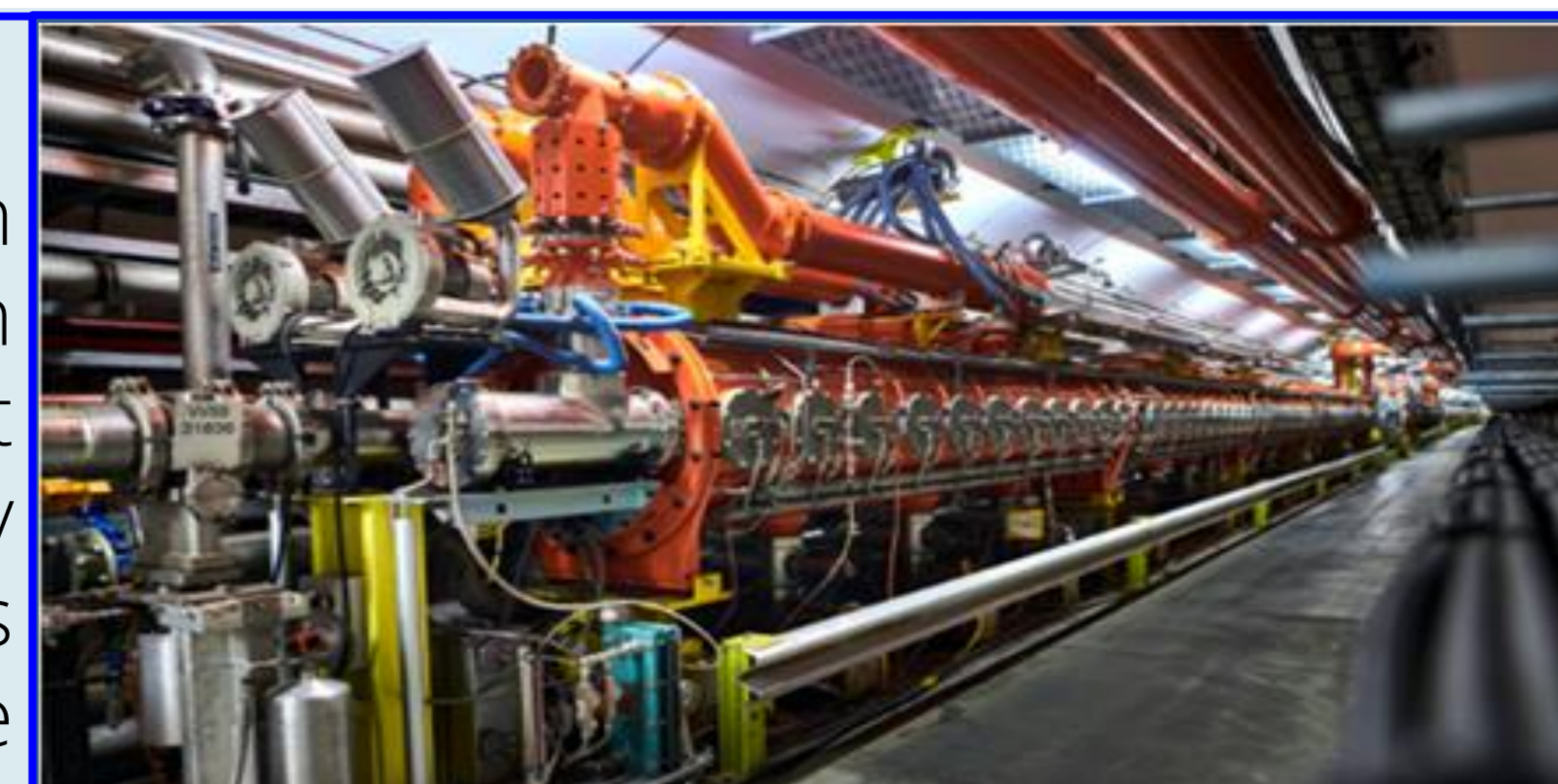
Fig 0. The SPS accelerating structure. [2]
