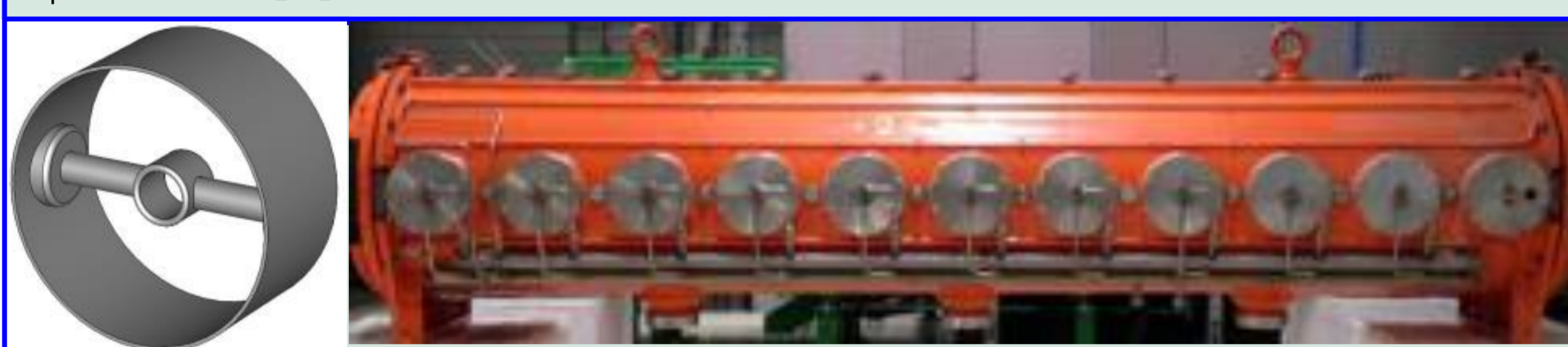
Fig 2. A 11-cell, parallel stem, accelerating section. [2]
