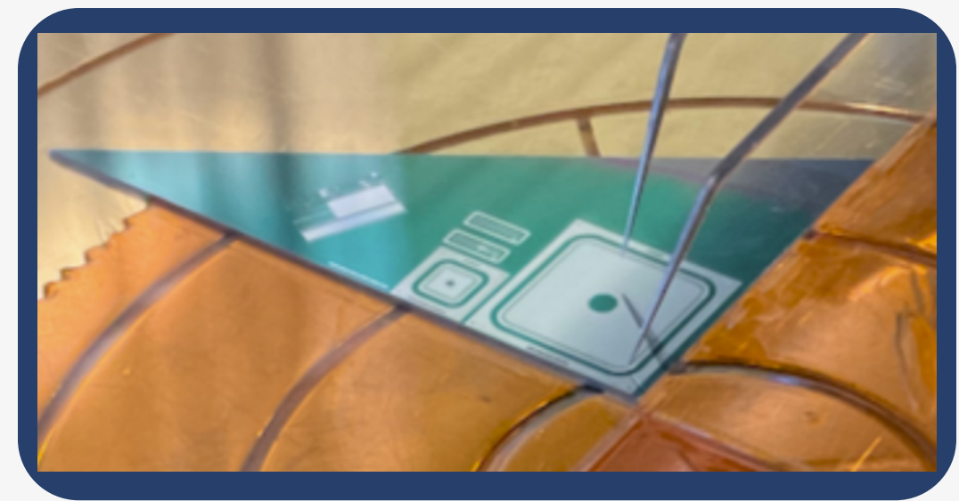
Contact is done with the DUT at the pad and at the guard ring
