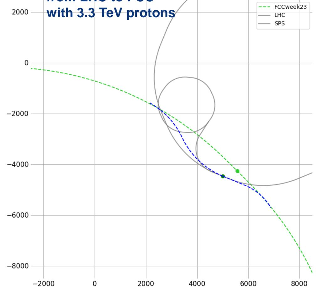
From 6 or 20 GeV Linac on Preveessin site, 1.7 km tunnel down to SPS LSS4, both particle species; then beam separation: (1) one beam into TI 8 tunnel and at LHC level a new tunnel of 1.8 km to connect to the FCC collider, (2) other beam fed through the SPS tunnel, extracting at LSS6 followed by short 800 m tunnel to connect to FCC; all lines from SPS level onwards compatible with 1.3 TeV protons; options also compatible with SPS as lepton pre-booster if 6 GeV linac.
