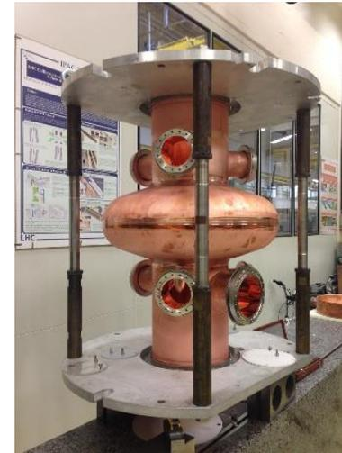
**400 MHz SRF cryomodule,**
