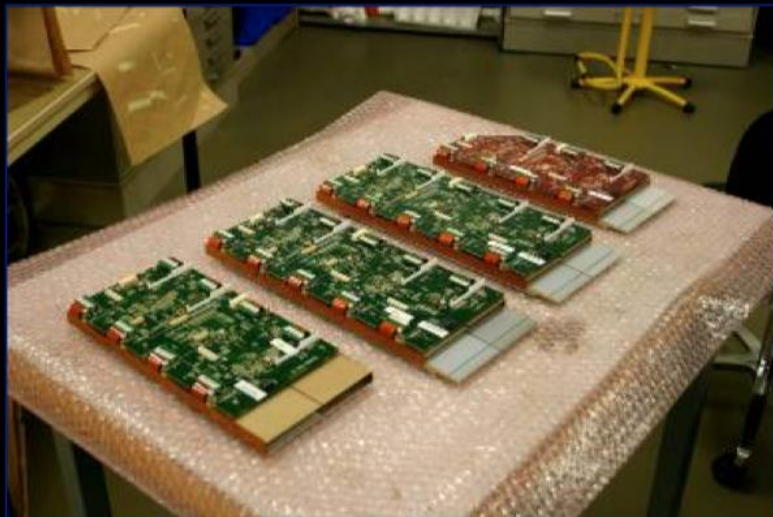
3 types of "ladder" filled with Si sensors
