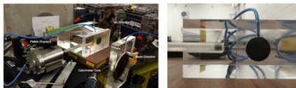
Calorimeter and ROOS chamber, Nat. Phys. Lab. UK (A. Subiel et al.)
