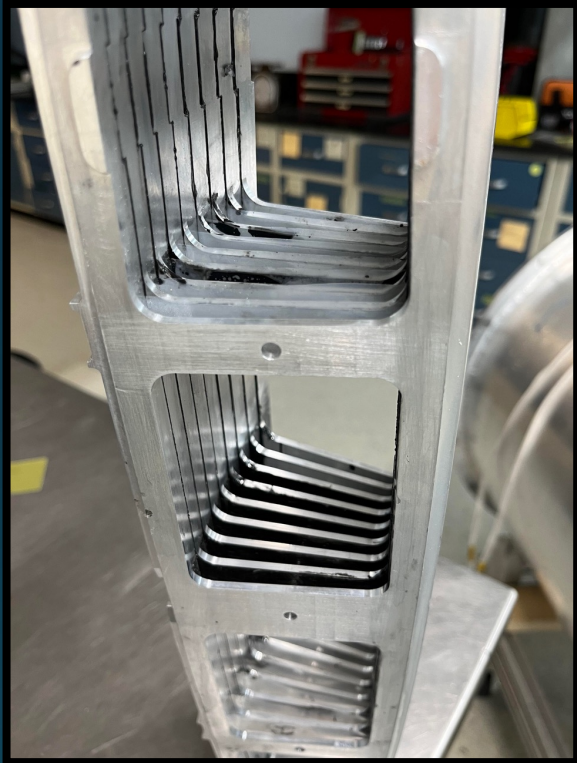
Magnet mandrel and winding (Superconducting Systems, Inc.)
