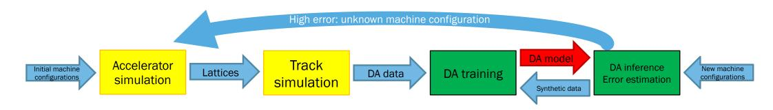
To keep the active framework functional, we continuously submit tracking simulations to generate new data for the ML model.
