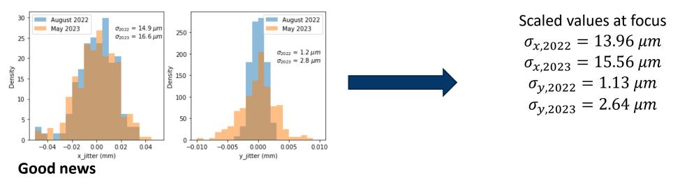
Comparing jitter measured in August 2022 and May 2023 no differences were observed in beam jitter:
