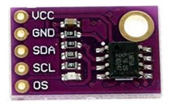
The LM75 board seems to have one more connection, the one labeled "OS", but we do not really need it. It is an output that the LM75 makes active whenever the temperature exceeds a set limit (so it can be used as a thermostat).
