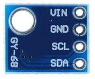
The BMP180 sensor board has four pins. We can connect them to our Arduino Nano as follows:
