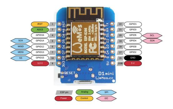
Note that pins have more than one denomination, depending whether you are using the Arduino IDE or MicroPython to program the CPU. In MicroPython, the GPIOxx number is used, so GPIO4 will be "Pin 4". The board has an LED, connected to GPIO pin 2 (also D4) so that the LED will be ON if the pin outputs 0, and off if the pin outputs 1.
