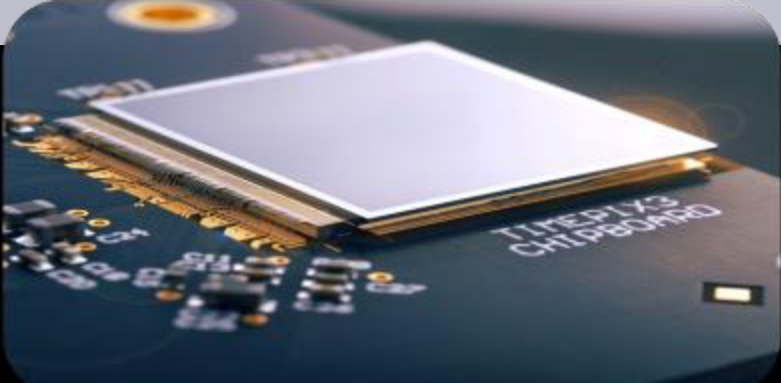
MEDIPIX Read-out chips for particle imaging
