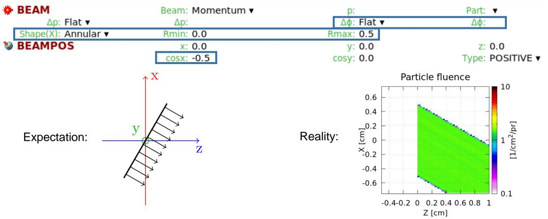
• Remember: the **BEAM** card sets the X-Y shape of the beam, which is not influenced by the beam direction set in the **BEAMPOS** card... so how can we rotate the beam?
