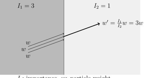
I: importance, w: particle weight Particle survives with probability  $I_2/I_1 = 1/3$ Surviving particle weight increased by  $I_1/I_2 = 3$
