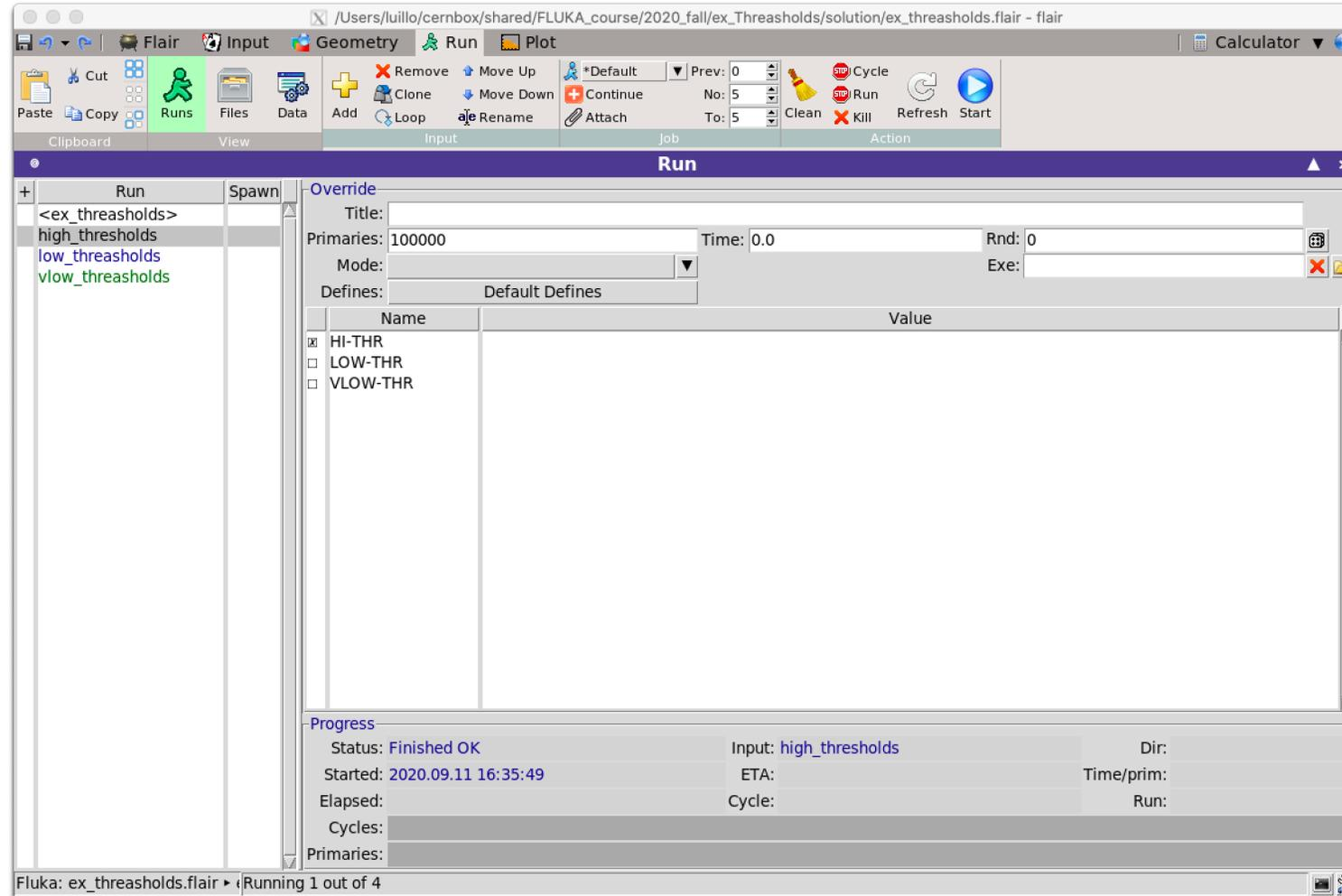
Run three simulations corresponding to high, low, or very low threshold values, with 5 cycles × 100000 primaries for each case
