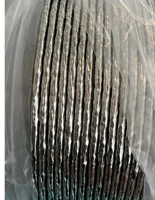
300-meter MgB 2 Cable
