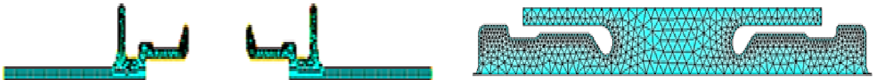
Element model and mesh for stress analysis of SS metal and GFRP section
