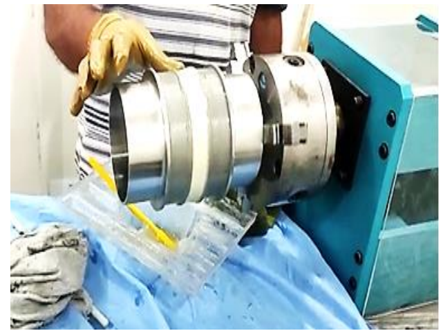
Fabrication by manual filament winding process
