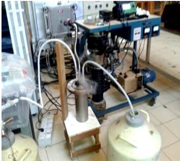
Schematic of He leak test at 77 K, 4.2 K
