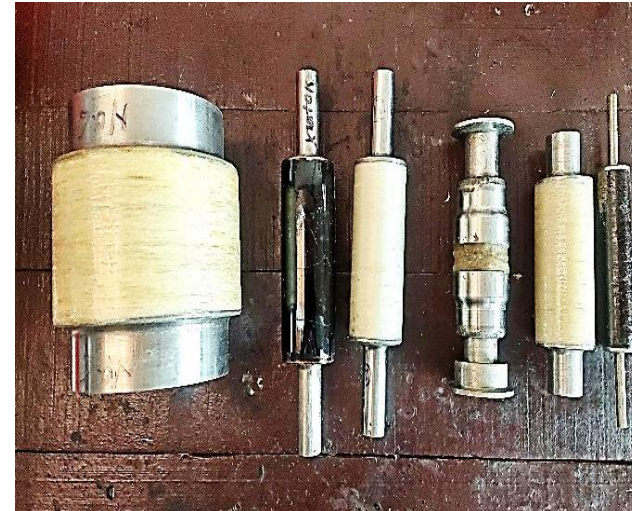
In-house fabricated various sizes of dissimilar material joints
