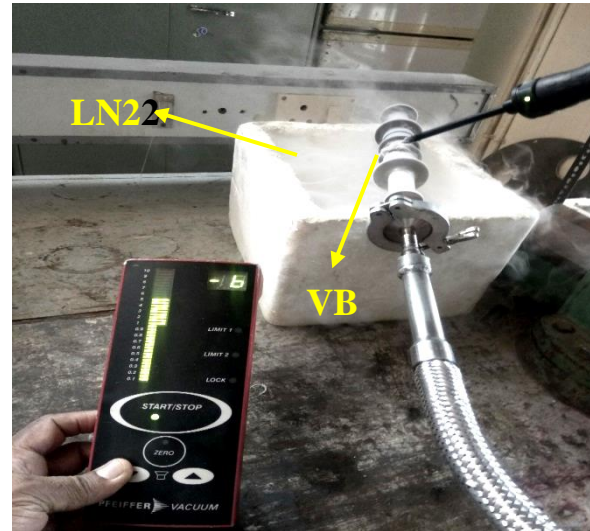
He leak test @ 10 bar LN2
