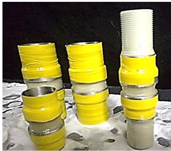
1 st stage bonding process
