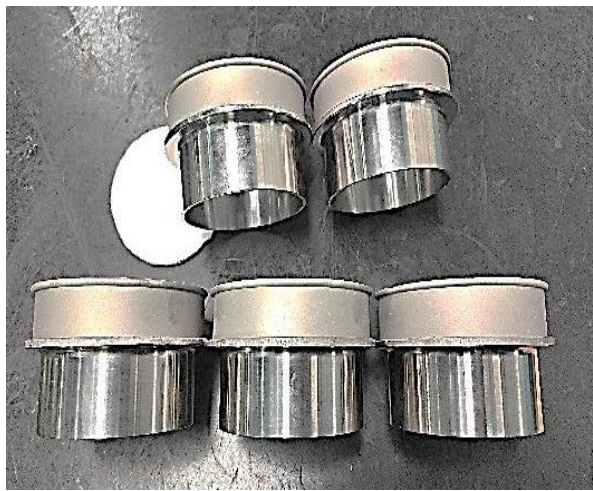
SS 316L sand blasted conductors
