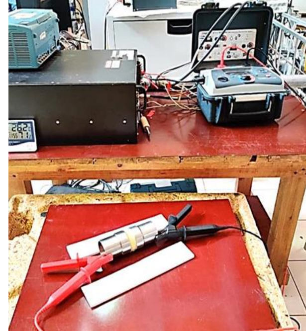
Electric DC Meggar test at 10 kV
