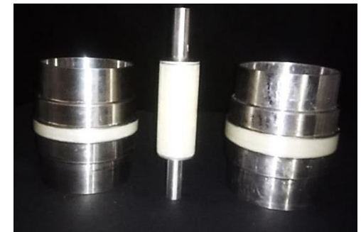
Glass fiber + SS dissimilar material joint (VB)
