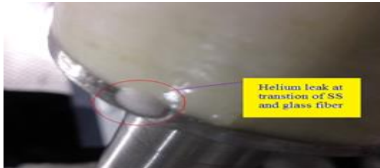
He leak after thermal cycle at 77 K
