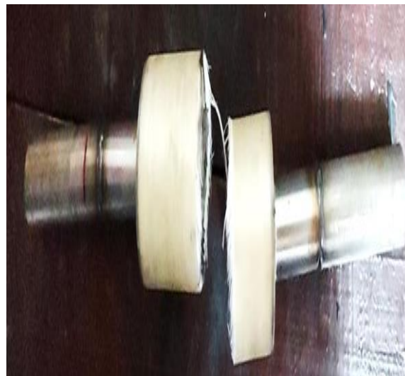
Fractured sample of SS+ GFRP material joint
