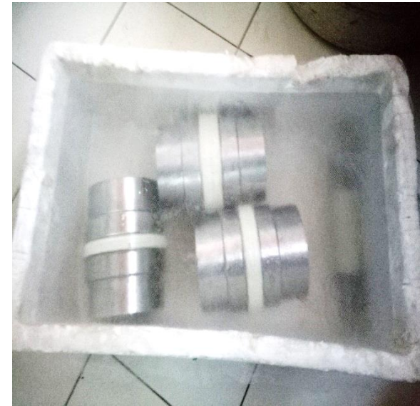
Thermal shock test at 77 K
