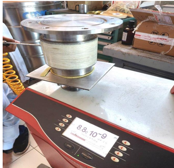
He leak test of VB at 300 K
