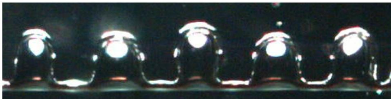
High speed visualization of film boiling
