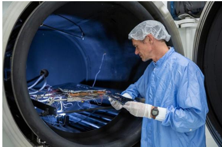
MLI testing Courtesy of NLR
