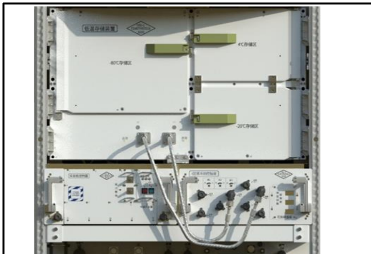
Cryogenic Storage Device in the Chinese Space Station 193 K-277 K
