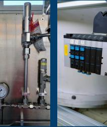
Buffer volumes to stabilize the two-phase flow, passive mechanical safety devices and (pneumatic) fail-save values help a lot
