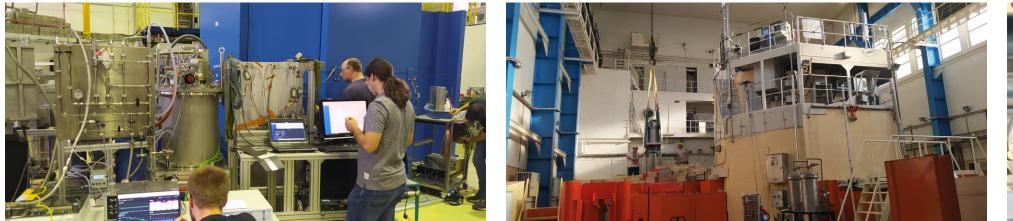
Operating the HBS cryostat for three beam times using a virtual server-based control system, database and HMI providing LH2 to a cold neutron moderator. Over 850 hours of failure-free operation in the radiation protection area.
