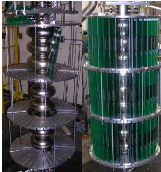
Array temperature measurement*
