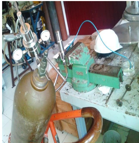
Testing of safety valve
