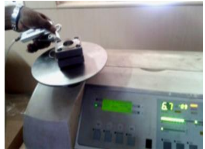
Rupture disc seal and He leak testing
