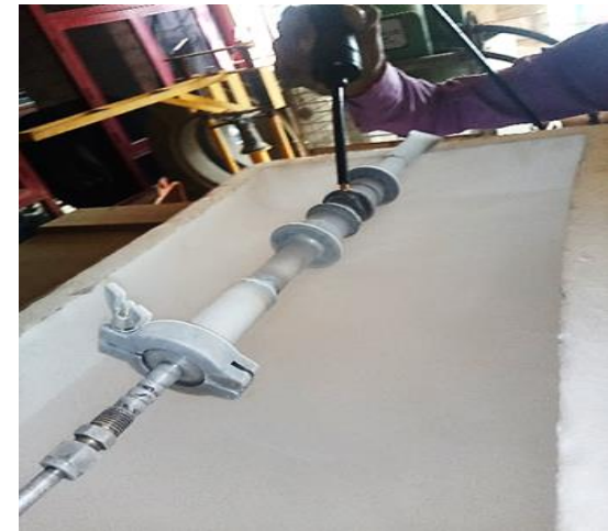
Thermal shock test of Flexible Hoses & He leak test of VB at 12 bar (g), 77 K
