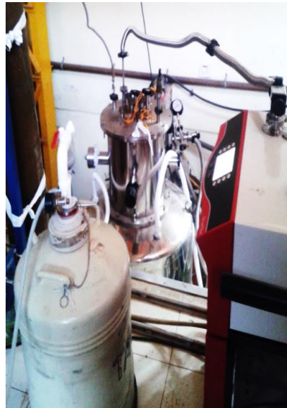
He leak test at 77K, 4.2 K, 0-20 bar of IB, Indium seal test Hydro test of Bellows at 20 bar
