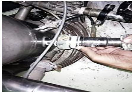
High pressure cryo grade thread sealant used in Helium connectors, Rupture disc coupler
