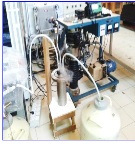
He leak test at 77K, 4.2 K, 0-20 bar of IB, Indium seal test Hydro test of Bellows at 20 bar
