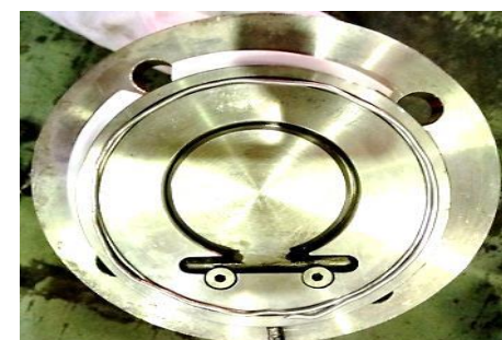
High pressure cryo grade thread sealant used in Helium connectors, Rupture disc coupler
