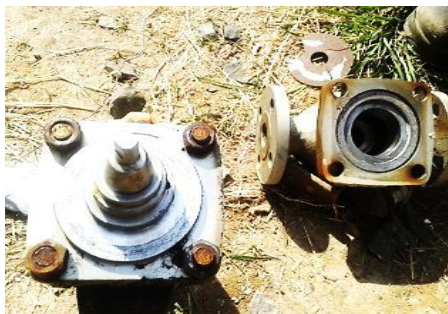
High pressure v/v developed seal, ANSI 150 Flange 'O' ring and gasket sealing at 16 bar(g)
