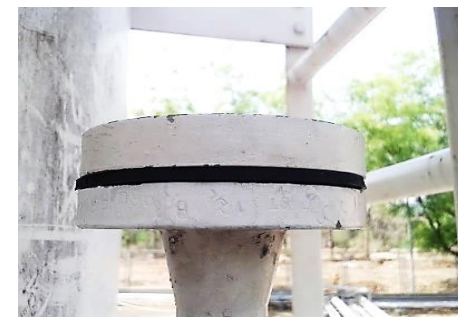
High pressure v/v developed seal, ANSI 150 Flange 'O' ring and gasket sealing at 16 bar(g)
