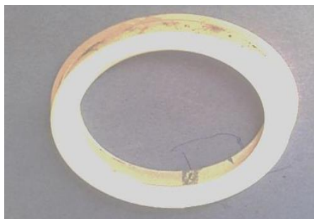
High pressure v/v developed seal, ANSI 150 Flange 'O' ring and gasket sealing at 16 bar(g)
