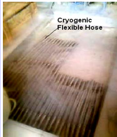
Thermal shock test of Flexible Hoses & He leak test of VB at 12 bar (g), 77 K
