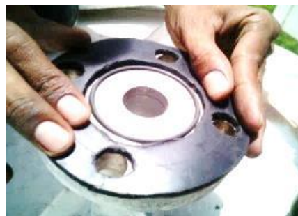
High pressure v/v developed seal, ANSI 150 Flange 'O' ring and gasket sealing at 16 bar(g)
