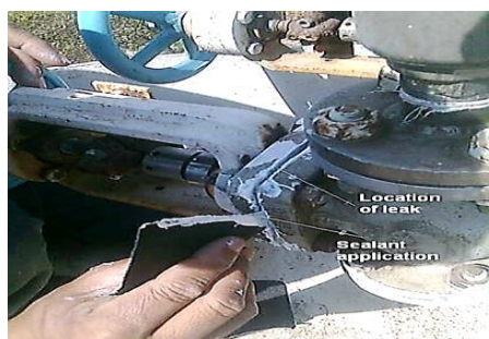
High pressure cryo grade thread sealant used in Helium connectors, Rupture disc coupler
