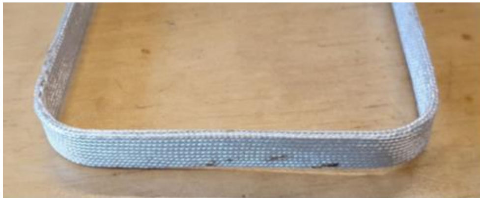
Sample 4: mullite insulation, some stains visible (possible leakage)
