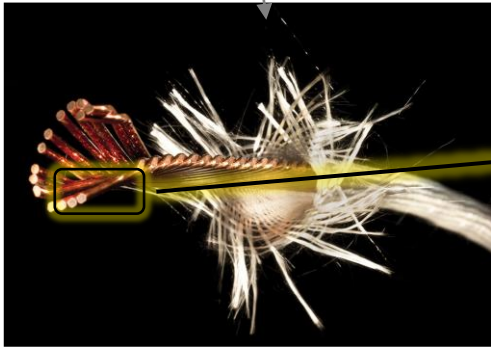
Unreacted Nb 3 Sn Rutherford cable, with S2 fibre glass insulation
