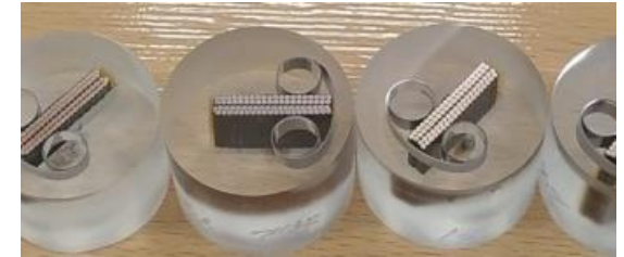
Embedded specimens – transverse cross sections
