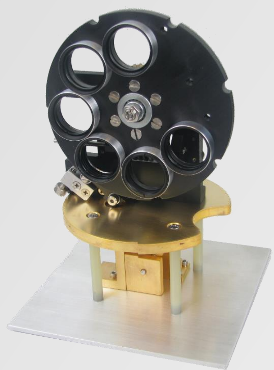
Fig 1. Example filter wheel assembly controlled by motor with position feedback from mechanical switches
