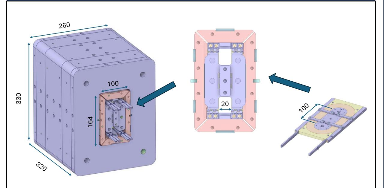
On the right a racetrack coil. In the centre, four coils are placed inside the intermediate support plates to form a common coil configuration. Then the system is inserted in the iron cavity and the cold mass is completed (on the left). In this configuration, the field in the centre of the two cavities is about 5 T.
