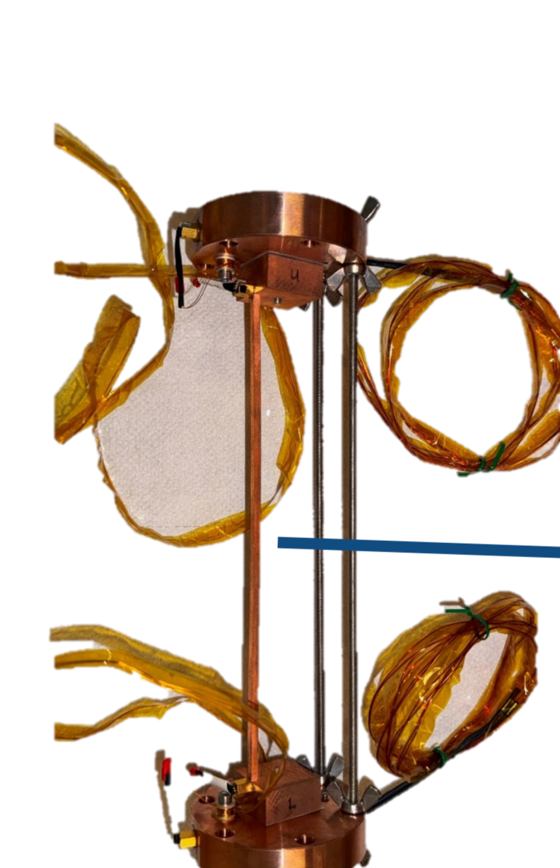
Specimen with heater blocks, thermometers and temporary support rods.
