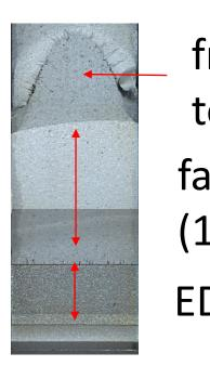
fracture toughness test fatigue crack (10-26mm)EDM notch (10mm)
