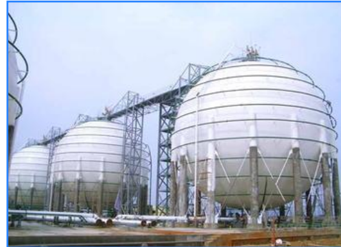
Cryogenic spherical storage tank Insulation material: polyurethane, glass wool
