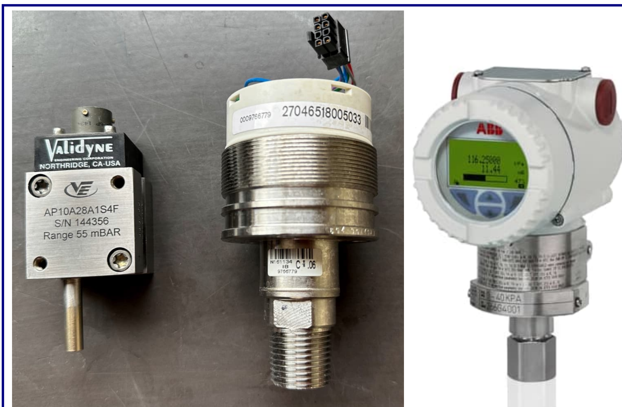
Pressure sensors under test: Valdyne AP 10 and ABB passive cell. Both have a 60 mbar range.
