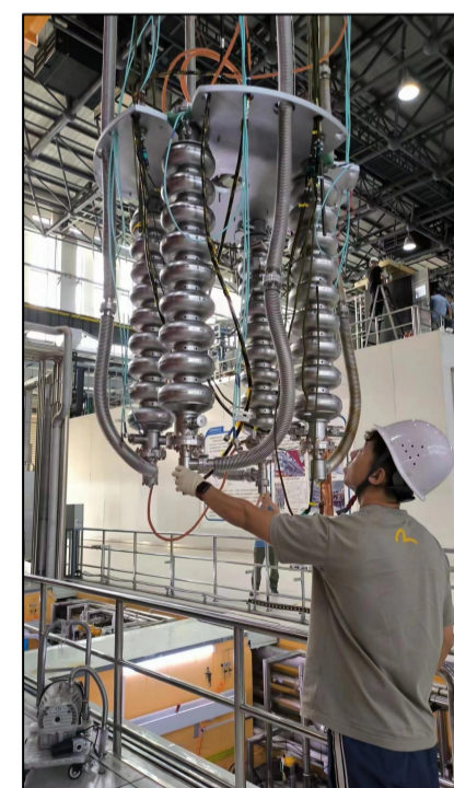
▲ Photo of VTS & four 1.3 GHz 9-cell cavities installed for VT
