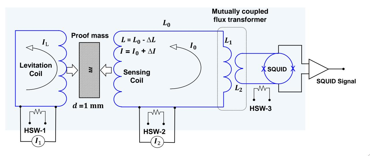
• Design of the SSG measuring apparatus and superconducting housing
