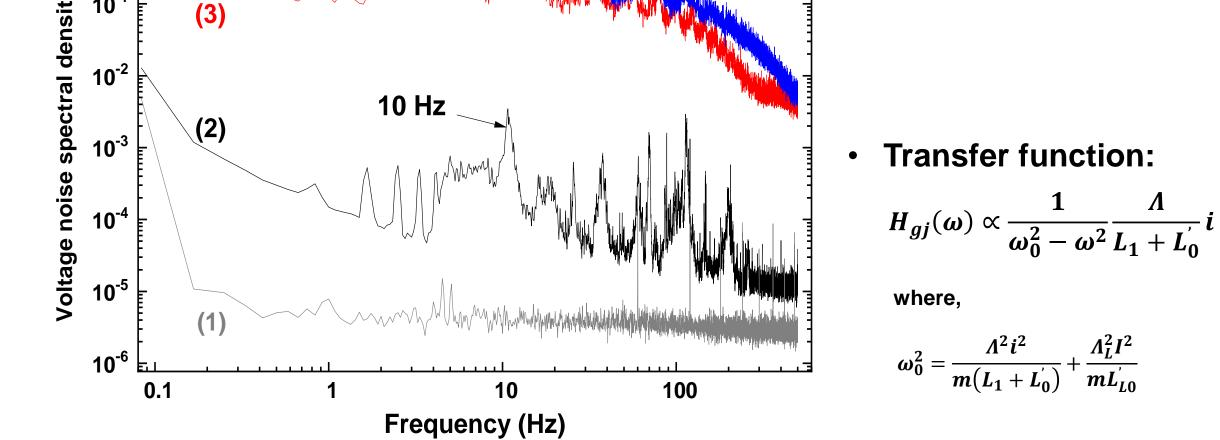
• Comparison of the survey spectrum of gravity for 16 hours
