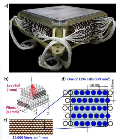
Figure 4: (a) AMS Electromagnetic Calorimeter. It is  $17 X_0$ . (b) Small section of a super layer of the ECAL. (c) Scintillation Fibers. (d) A cell which is collected by the one of anode of the PMT [1].
