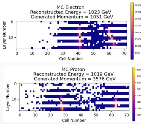
Figure 5: ECAL shower signals. When the electrons and protons pass through the electromagnetic calorimeter, many secondary particles are created. The particles deposits energies which are recorded by the photomultiplier tubes.
