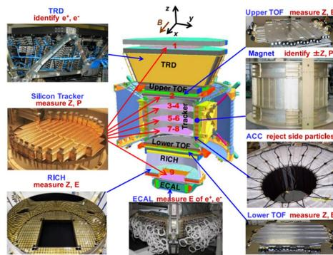
Figure 2: AMS detector with the subdetectors [1].
