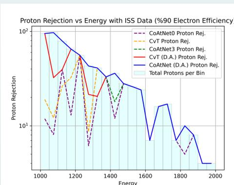
Figure 10: Proton Rejection vs. Energy at 90% Electron Efficiency with ISS Test Dataset.
