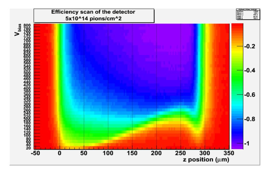
Back of the detector becomes more efficient than front region at high voltages
