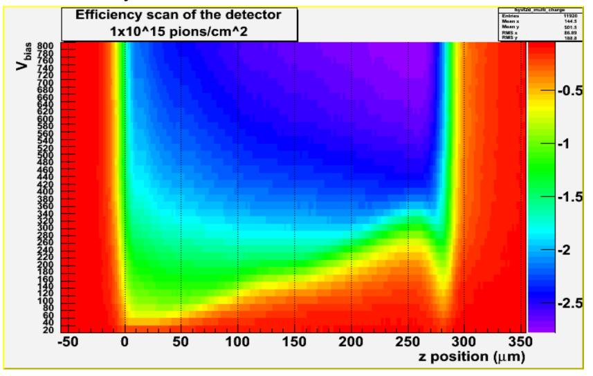
Again, more efficiency in the back region at high voltages. Trapping is influencing less carriers generated in this region (might be due to higher drift velocity of electons that have anyway lifetimes comparable to holes)
