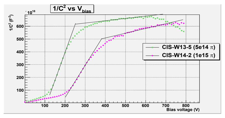
Depletion voltages from CV(-25C, 55 Hz) and IV:
