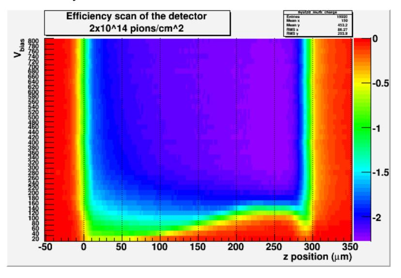
Back of the detector becomes more efficient than front region at high voltages
