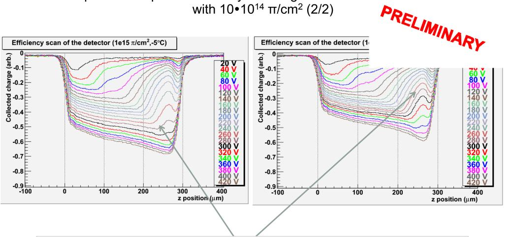
At -5° C, at 300 V, signs of underdepletion at 280 V. At 10° C, detector is clearly underdepleted at 280 V. Depletion achieved @ 380 V
