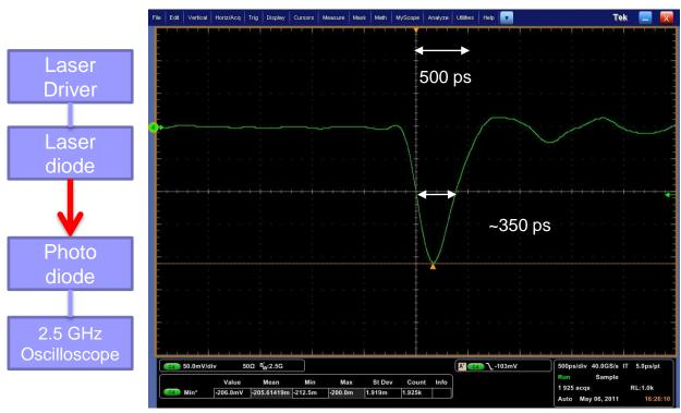
Parameters of the laser as measured with photodiode (real parameters are probably better)
