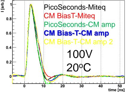
W336 diode, FZ n-type, 2 kΩcm,  $V_{fd}$ =180, electron injection – front ill., laser 1.4 ns FWHM
