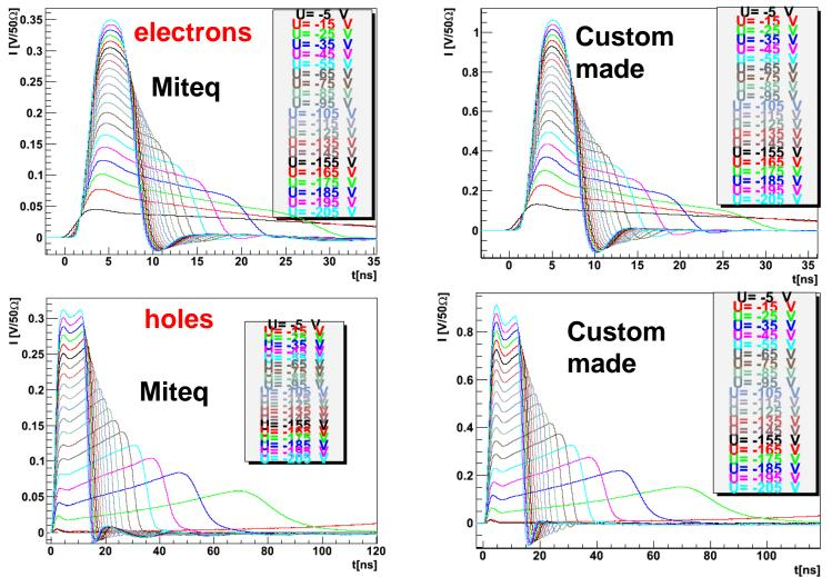
Electron injection – almost equal response apart from the difference in amplification (factor of 3)
