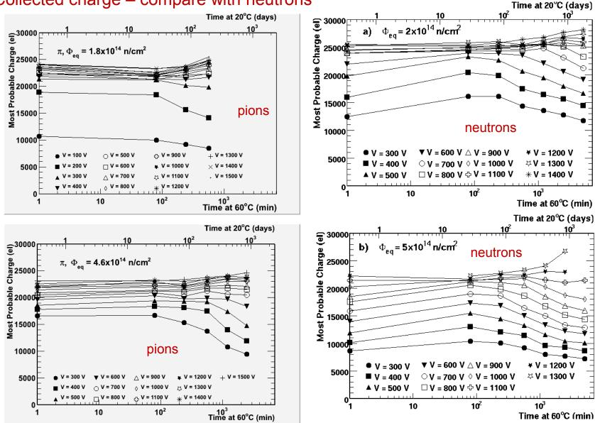
→Similar behaviour for pions and neutrons at high voltage (except at the highest voltage for neutrons)
