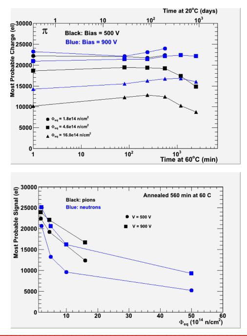
at low voltages higher charge collected after irradiation with pions than after neutrons
