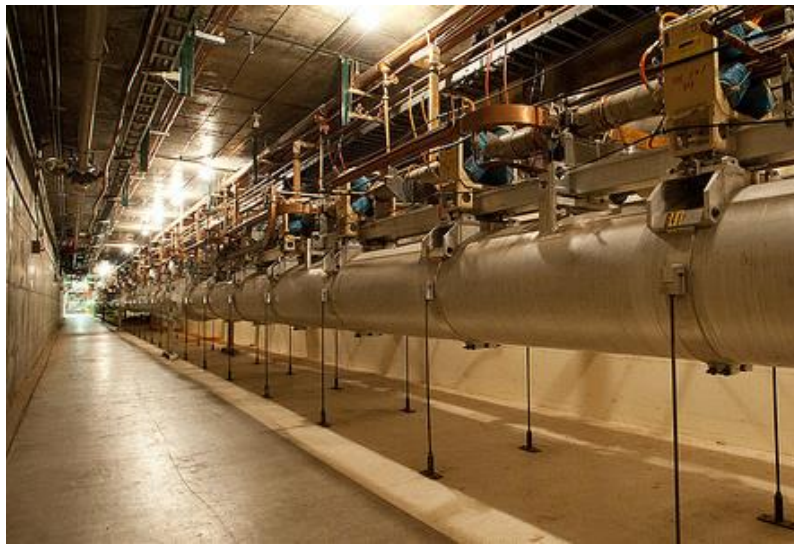
The 3 km Stanford Linear Accelerator ; 2.8 GHz normal conducting cavities
