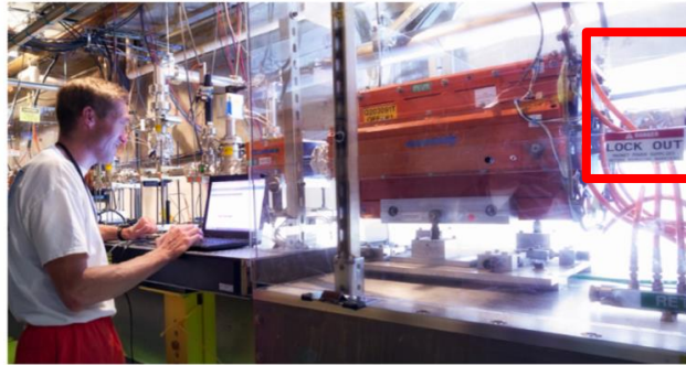
a) Normal conducting magnetic focusing quadrupole at the FACET high energy test facility
